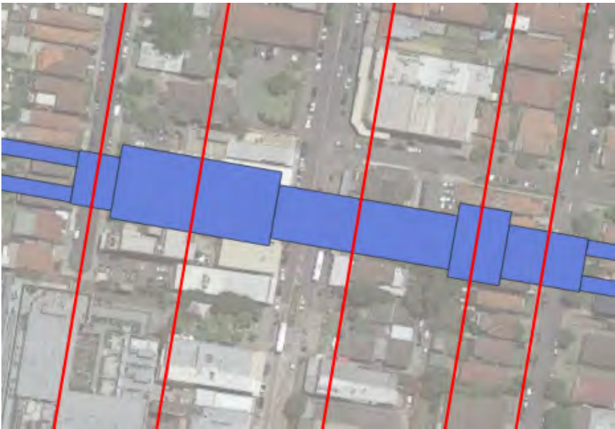
FIGURE 2 GROUND PROFILES CONSIDERED IN FIVE DOCK STATION SEEP/W CROSS SECTION MODEL (SECTION LINES IN RED)
