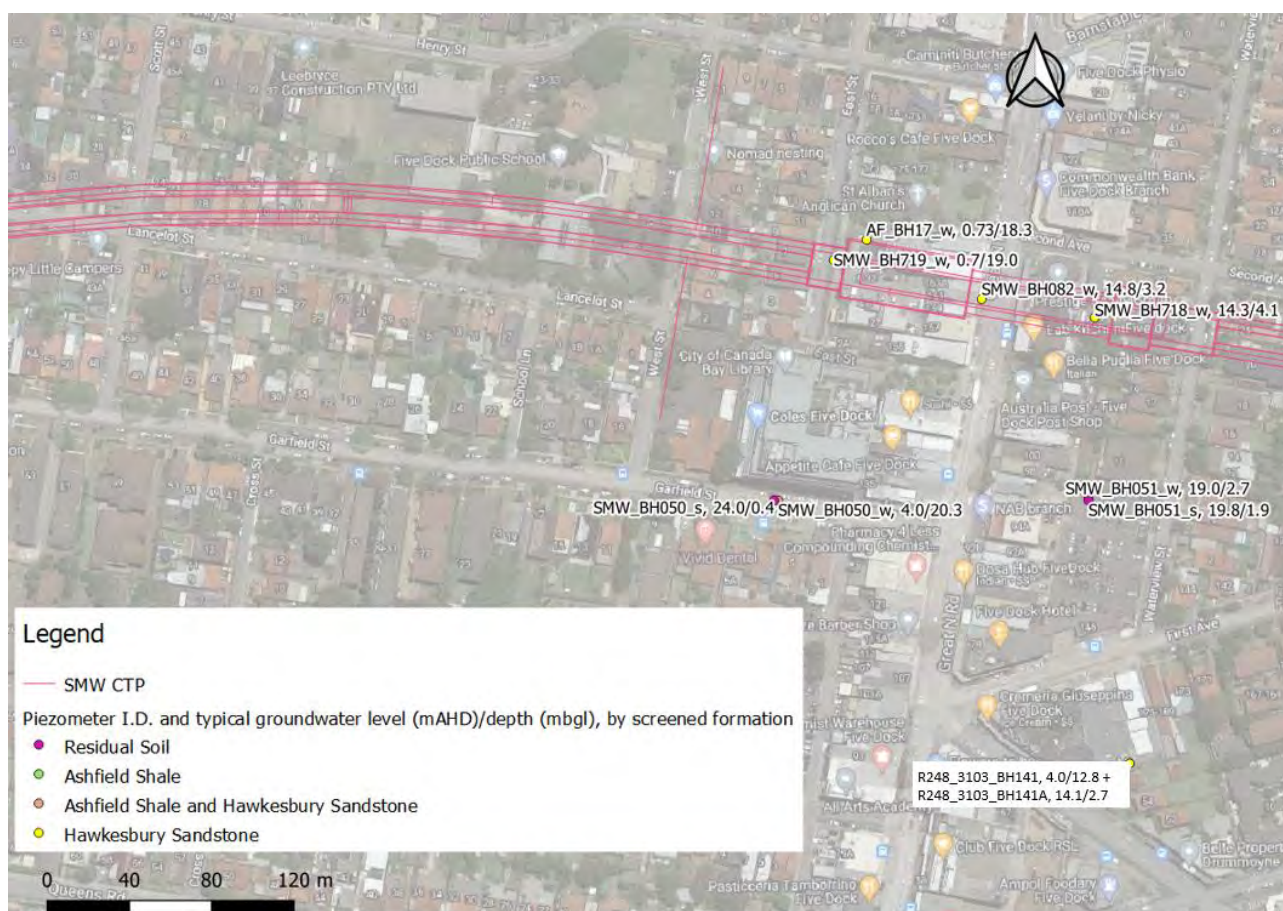
FIGURE 3 - GROUNDWATER LEVELS AT FIVE DOCK STATION
