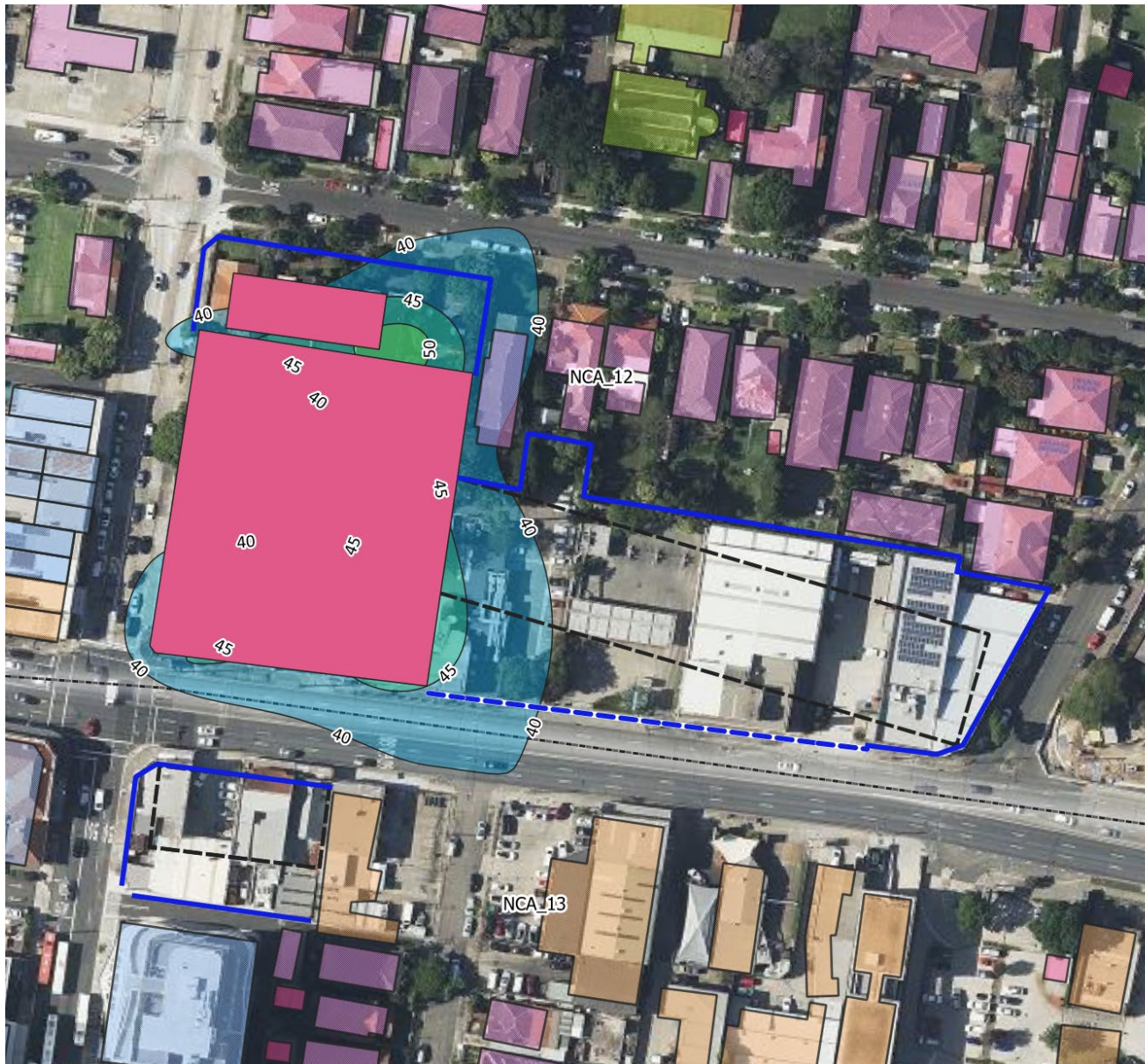
TBM Re-launch Burwood Noise Contours - All Hours Shed doors closed
