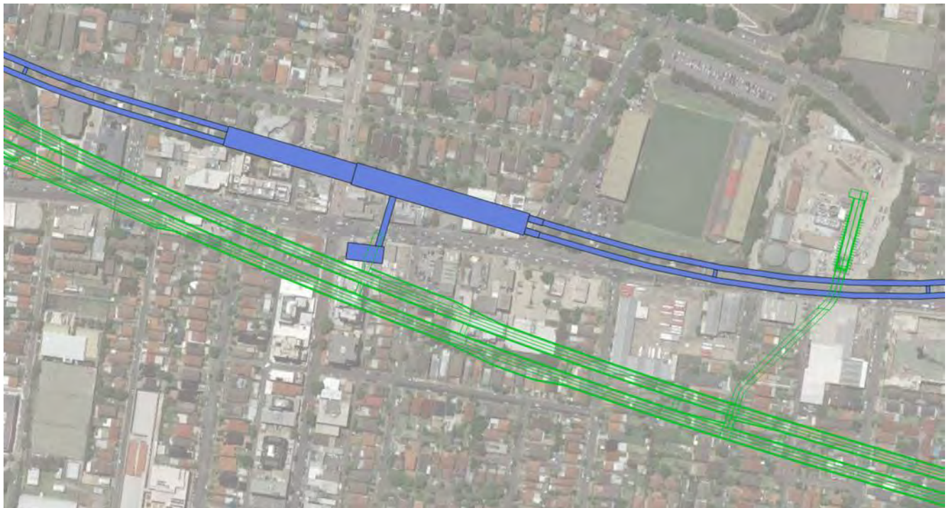
FIGURE 4-6: LOCATION OF BURWOOD NORTH STATION BOX, CAVERN AND SHAFT (IN BLUE); AND M4 EAST TUNNELS, SUBSTATION NO. 5 AND CINTRA DECLINE (IN GREEN)
