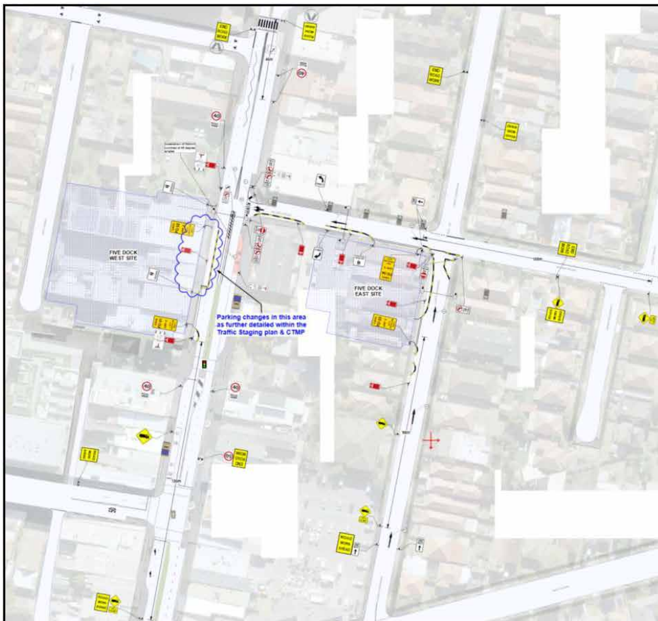
FIGURE 7: OVERVIEW OF LONG TERM TRAFFIC STAGING
